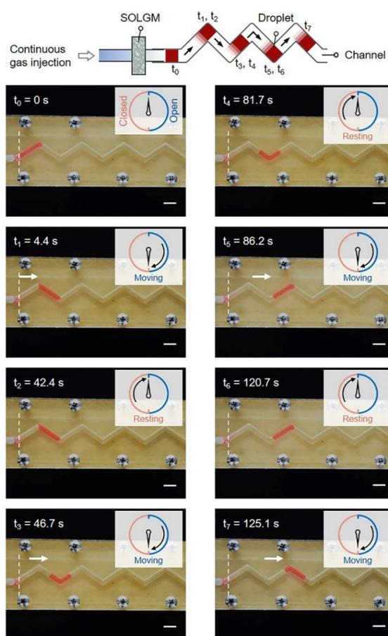
**Figure 5.** Demonstration of SOLGM for periodic gas transport in droplet microfluidics. The droplet is deionized water dyed with magenta filling ink. White dotted lines represent the initial position of the droplet movement. Scale bars: 10 mm.
