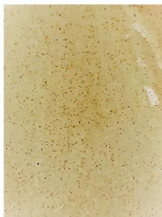
**Figure 14.** Photo showing the homogeneous distribution of the added  $\text{Fe}_{20}\text{Ni}_{80}$  magnetic alloys embedded inside the cellulose acetate (CA) polymer matrix.
