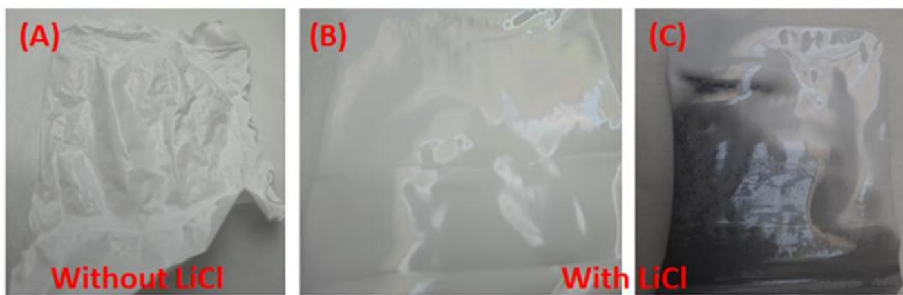
**Figure 2.** Photos illustrating the effect of the addition of lithium chloride (LiCl) on shrinkage in the prepared blank cellulose acetate (CA) and magnetic mixed CA matrix membranes after drying in atmospheric air. The blank CA without (A) and with (B) LiCl and the magnetic mixed CA matrix membrane with LiCl (0.1 wt.%) (C).
