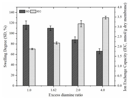
Figure 7. The effect of excess diamine ratio on SD and IEC of synthesized AEMs (BR:1.07).
