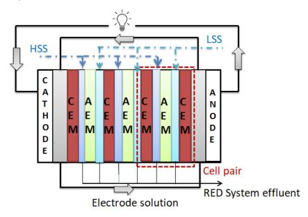
**Figure 1.** Schematic of a RED system (HSS: High saline solution, LSS: Low saline solution) (Adapted from [9]).
