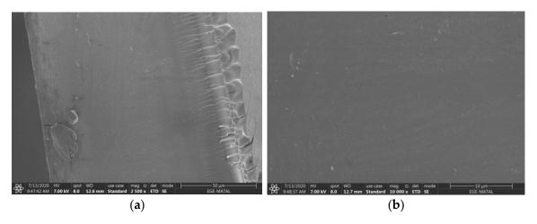
**Figure 5.** Cross-section SEM images of ER4-BR1.07 AEM (a) 2500×, (b) 10,000×.
