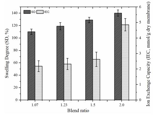
Figure 8. The effect of blend ratio on SD and IEC of synthesized AEMs (ER:1.62).
