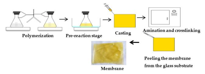
Figure 2. Preparation procedure of AEMs.
