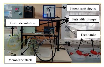
**Figure 4.** RED system components.
