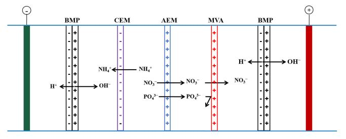
**Figure 1.** Schematic diagram of experimental equipment. CC: cathode compartment; AWC: ammonia compartment; WWC: wastewater compartment; PC: phosphate compartment; NAC: nitric acid compartment; AC: anode compartment.
