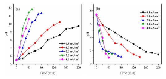
Figure 5. Effect of current density on (a) solution pH of ammonia compartment and (b) nitric acid compartment.
