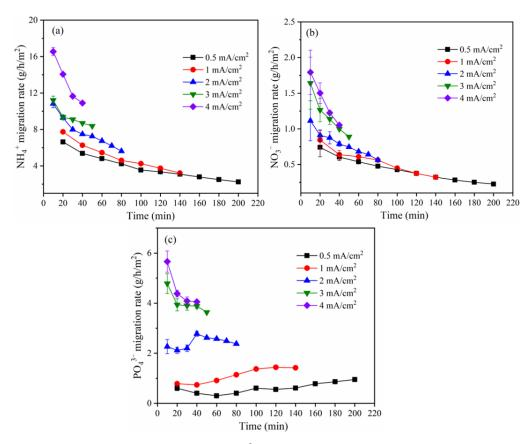
**Figure 8.** Migration rate of (a)  $NH_4^+$ , (b)  $PO_4^{3-}$ , and (c)  $NO_3^-$  under different current densities.
