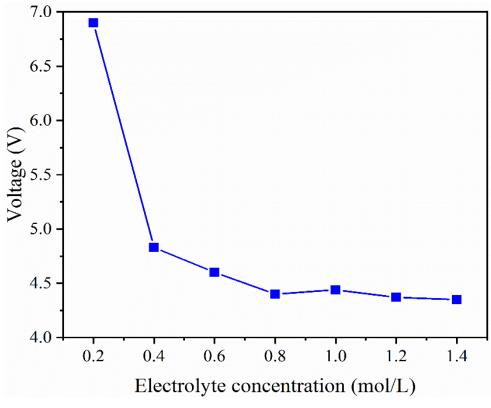
Figure 2. Cell voltage variation of cell voltage with Na<sub>2</sub>SO<sub>4</sub> concentration.
