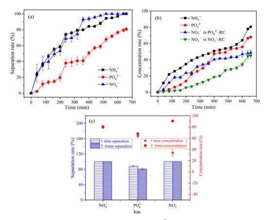
**Figure 7.** (a) separation and (b) concentration of  $NH_4^+$ ,  $PO_4^{3-}$  and  $NO_3^-$  with the volume ratio of  $V_{WWC}/V_{AWC}$ ,  $V_{WWC}/V_{PC}$ , and  $V_{WWC}/V_{NAC}$  was 5:1 and (c) the comparison with volume ratio of  $V_{WWC}/V_{AWC}$ ,  $V_{WWC}/V_{PC}$ , and  $V_{WWC}/V_{NAC}$  was 1:1.
