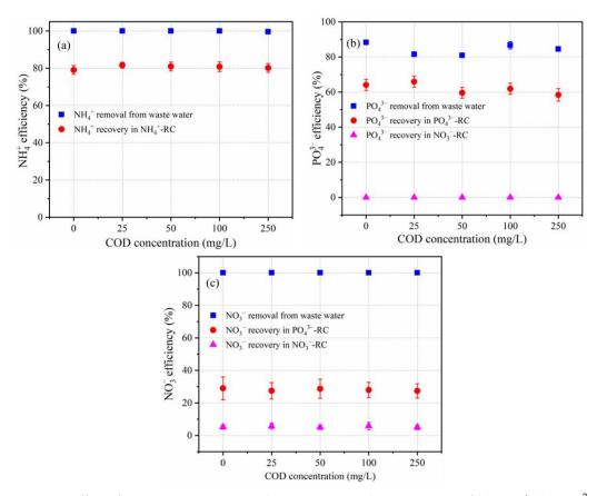
**Figure 6.** Effect of COD concentration on the separation and concentration of (**a**)  $NH_4^+$ , (**b**)  $PO_4^{3-}$  and (**c**)  $NO_3^{-}$ .
