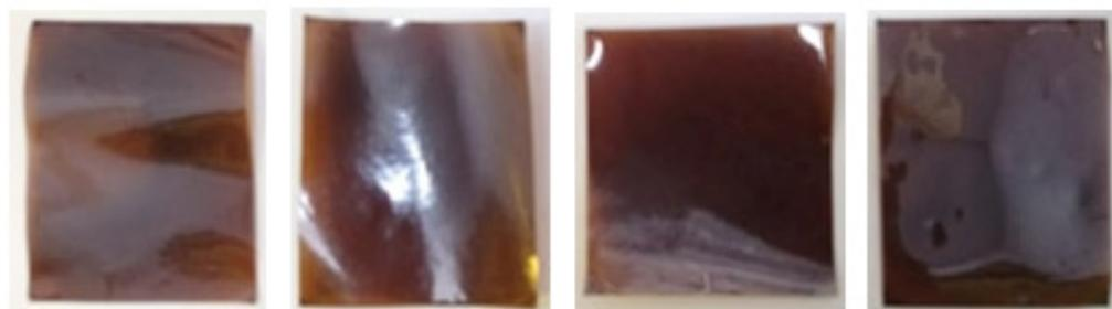
**Figure 1.** Photo of SPPQ films with sulfur content 2.6, 4.2, 5.5, and 7%.
