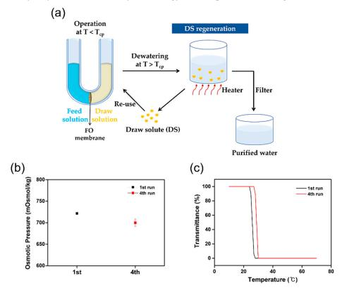
**Figure 9.** Recyclability study of [TBP][DMBS] in four cycles: (**a**) scheme of the FO system, (**b**) osmotic pressures, and (**c**) thermoresponsive behavior tests. From the 2nd to the 4th run, the recovered [TBP][DMBS] from the previous run was used.
