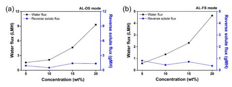
**Figure 8.** Water and reverse solute flux of tetrabutylphosphonium 2,4-dimethylbenzenesulfonate ([TBP][DMBS]) according to the concentration at room temperature in (**a**) AL-DS mode and (**b**) AL-FS mode.
