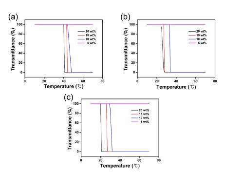
**Figure 7.** Transmittance curve of tetrabutylphosphonium (**a**) 4-methylbenzenesulfonate ([TBP][MBS]), (**b**) 2,4-dimethylbenzenesulfonate ([TBP][DMBS]), and (**c**) 2,4,6-trimethylbenzenesulfonate ([TBP][TMBS]) according to the temperature change.
