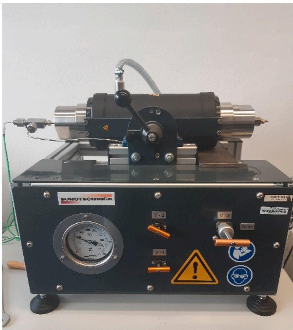
**Figure A1.** Tilting high-pressure vessel (280 mL, Eurotechnica GmbH, Germany).
