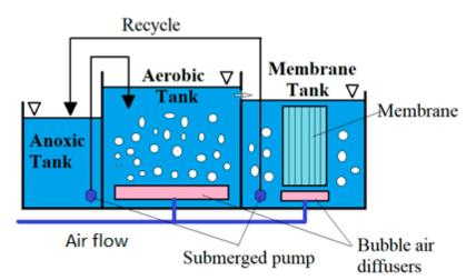
Figure 1. Wastewater treatment in MBRs (membrane biological reactor) (own study).
