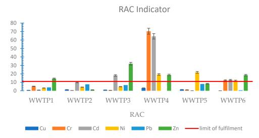
Figure 5. RAC indicator of heavy metals in sewage sludge.
