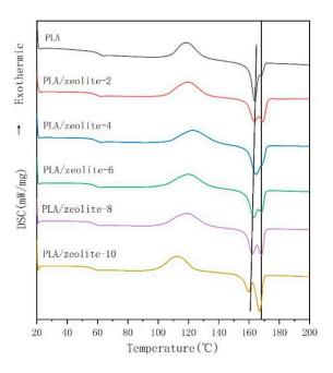
Figure 5. DSC second heating curve of PLA and PLA/zeolite composites.
