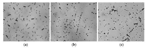
**Figure 6.** The polarizing microscope photographs of PLA/zeolite-4 (**a**), PLA/zeolite-6 (**b**) and PLA/zeolite-8 (**c**) amplified 100 times.
