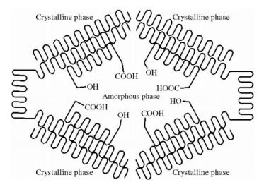
Figure 10. Schematic depiction of solid-state polycondensation.
