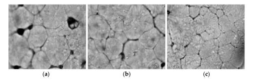
**Figure 7.** The polarizing microscope photographs of PLA/zeolite-4 (**a**), PLA/zeolite-6 (**b**) and PLA/zeolite-8 (**c**) amplified 1000 times.
