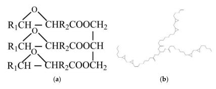
Figure 9. The skeletal structure (a) and stereoscopic structure (b) of ESO.
