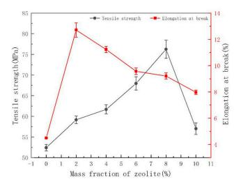
Figure 13. Effect of zeolite mass fraction on the mechanical properties of PLA composite films.
