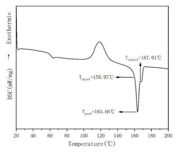
Figure 3. DSC second heating curve of PLA.
