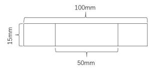
Figure 1. The size of the sample for the tensile strength test.
