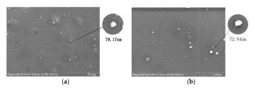
Figure 12. Dispersion size of zeolite in PLA/zeolite-2 magnified 2000 times (a) and 8000 times (b).
