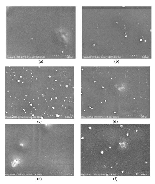
**Figure 11.** SEM images of PLA (**a**) and PLA/zeolite composites magnified 8000 times with different zeolite concentrations: (**b**–**f**) shows 2, 4, 6, 8 and 10 wt%, respectively.
