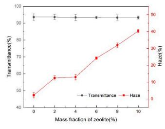
Figure 8. The effect of zeolite on the light transmittance and haze of PLA composites.
