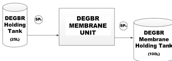
Figure 5. Membrane Bioreactor Unit Set-up. (SP=sample point).
