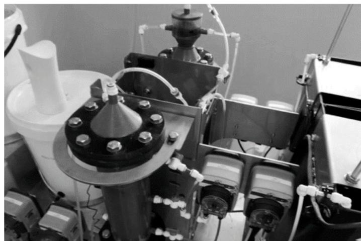
**Figure 1.** Lab-Scale Treatment Plant for PSW [21]—Reprinted from Membranes, vol 11, Meyo, H.B.; Njoya, M.; Basitere, M.; Ntwampe, S.K.O.; Kaskote, E., “Treatment of Poultry Slaughterhouse Wastewater (PSW) Using a Pre-treatment Stage, an Expanded Granular Sludge Bed Reactor (EGSB), and a Membrane Bioreactor (MBR)”. Copyright (2021), with permission from MDPI.
