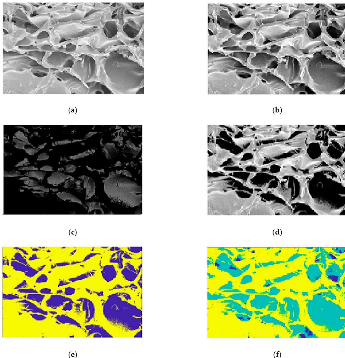
**Figure 8.** Classification: (Case1) Chitosan image origin (a), image enhanced (equalization) (b), classification cluster 1 (c), classification cluster 2 (d), K-means classification (2 classes) (e), and K-means classification (3 classes) (f).
