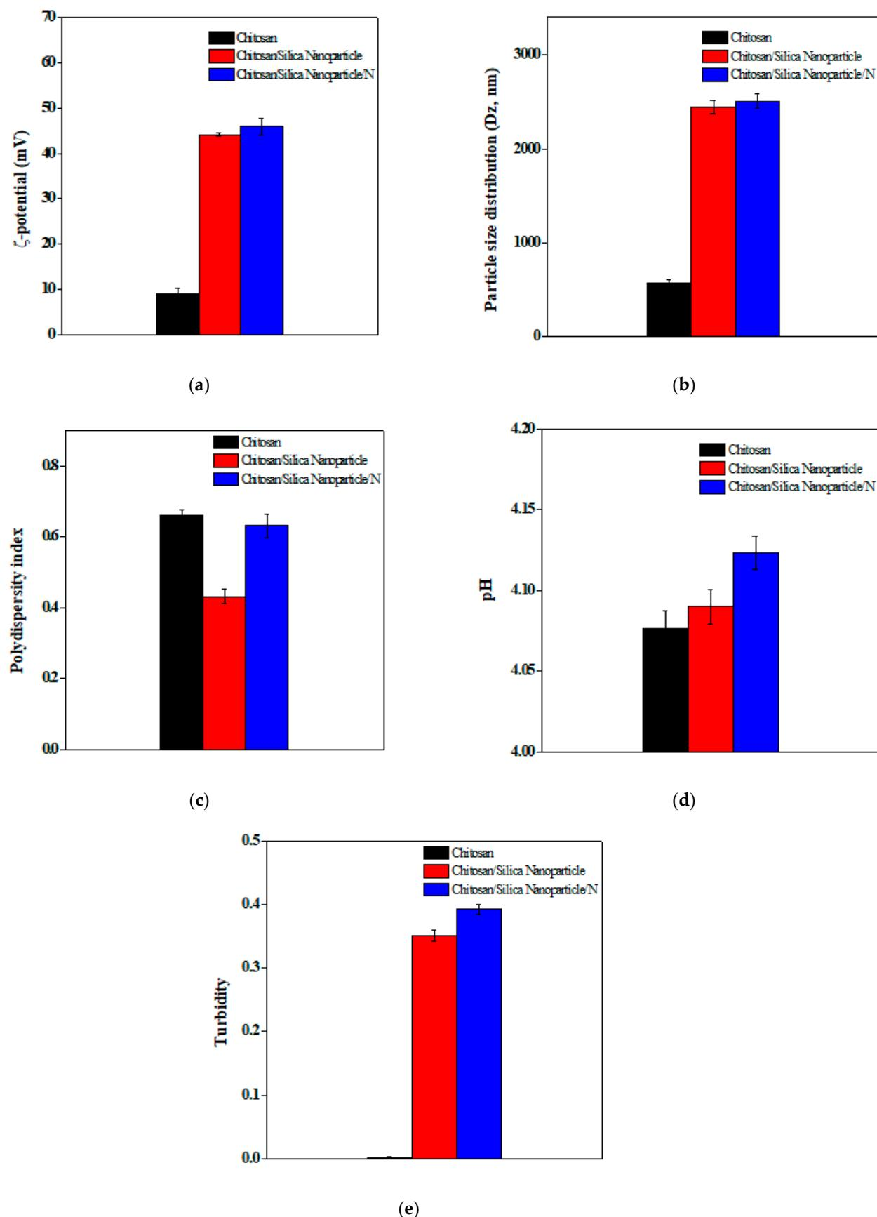
**Figure 5.** Some physical–chemical characteristics;  $\zeta$ -potential (a), particle size distribution (b), polydispersity index (c), acidity (d), and turbidity (e) of the novel films.
