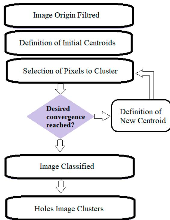
**Figure 3.** The flow chart of K-means clustering.
