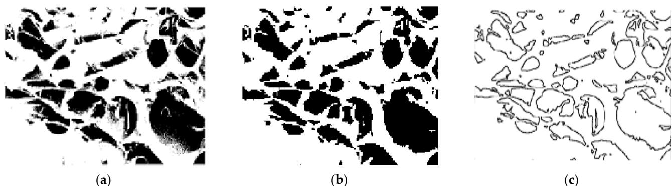
**Figure 10.** Segmentation by regions; image binarized without median filter (a), image filtered and binarized (b), and image segmented (c).
