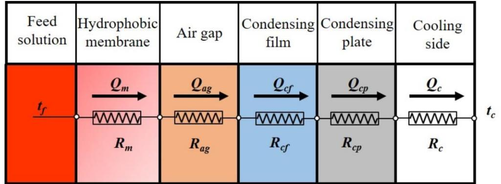
Figure 5. Schematic of heat transfer in ACMD process.
