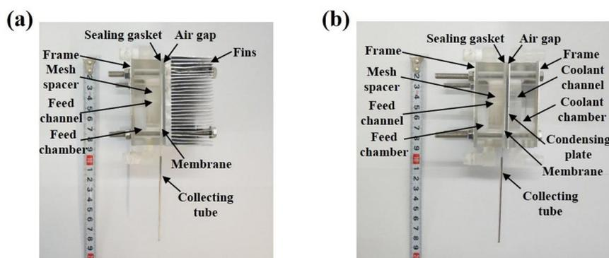
Figure 2. Photograph of the module used in this work. (a) ACMD module, (b) WCMD module.
