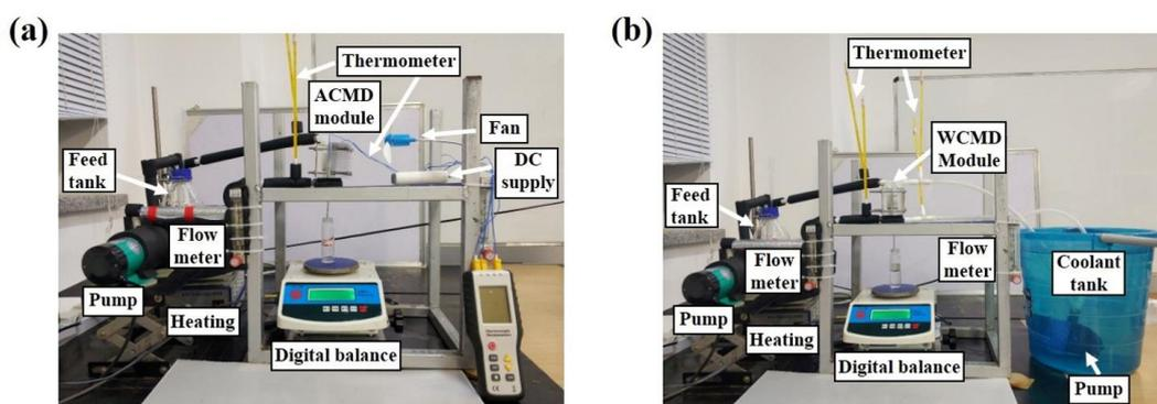
Figure 1. Photograph of the apparatus used in this work. (a) ACMD experimental apparatus, (b) WCMD experimental apparatus.
