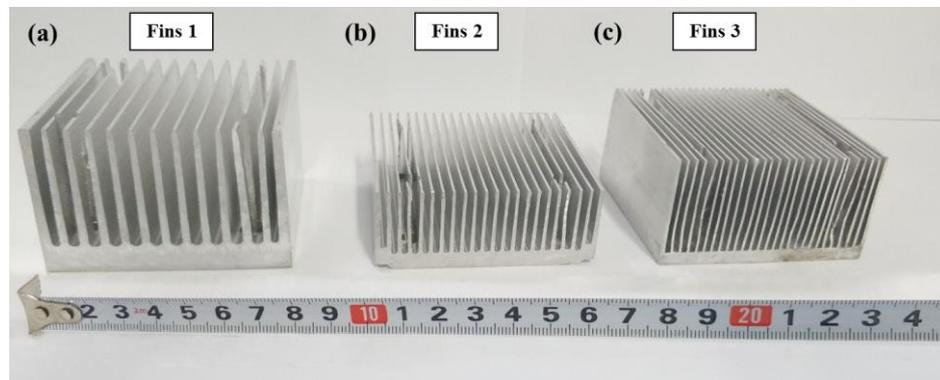
**Figure 4.** The aluminum finned condensing plates used in this work.
