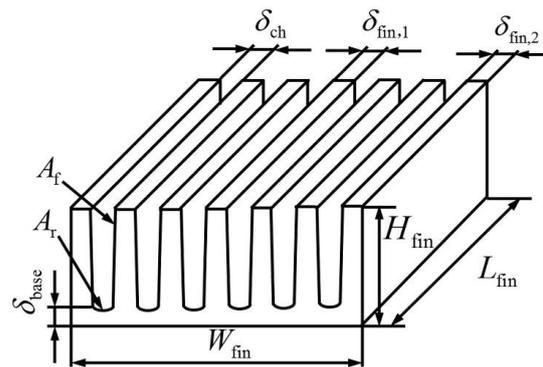
**Figure 3.** Schematic diagram of fins structure.  $L_{fin}$ : length of the fins;  $W_{fin}$ : width of the fins;  $H_{fin}$ : height of the fins;  $\delta_{ch}$ : the fin pitch;  $\delta_{fin,1}$ : the thickness of the inner fin;  $\delta_{fin,2}$ : the thickness of the outer fin;  $\delta_{base}$ : the thickness of the substrate;  $A_r$ : surface area of the substrate;  $A_f$ : side area of the fins.
