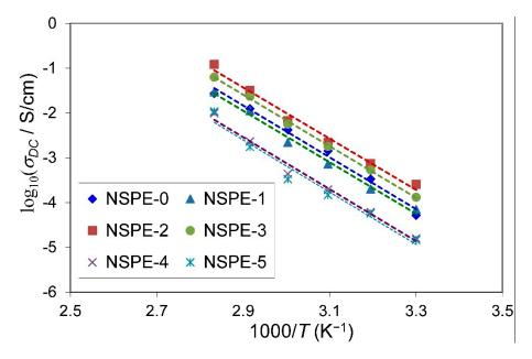
Figure 7. Temperature-dependent direct current (DC) conductivity for PVA/NH<sub>4</sub>NO<sub>3</sub>/ZnO NSPEs.
