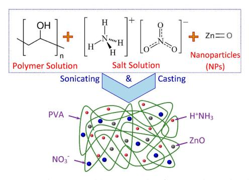
**Figure 1.** Sample preparation and characterization scheme for proton-conducting polyvinyl alcohol (PVA)/NH<sub>4</sub>NO<sub>3</sub>/ZnO nanocomposite solid polymer electrolytes (NSPEs).
