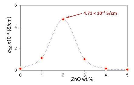
Figure 6. Ionic conductivity as a function of ZnO wt.% at room temperature.
