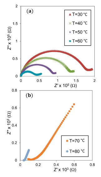
**Figure 5.** Impedance plot of the NSPE-2 sample at temperatures of 30–60  $^{\circ}$ C (**a**) and 70–80  $^{\circ}$ C (**b**).
