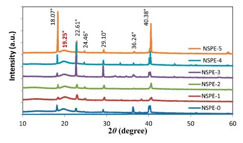
**Figure 2.** XRD pattern plots for PVA/NH<sub>4</sub>NO<sub>3</sub>/ZnO NSPEs with different ZnO-nanoparticle (NP) contents.
