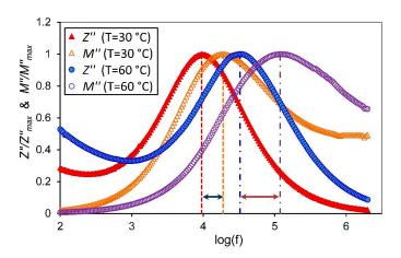
**Figure 9.** The change of normalized imaginary parts of impedance  $(Z'' / Z''_{max})$  and electric modulus  $(M'' / M''_{max})$  versus frequency at temperatures of 30 °C and 60 °C for the PVA/NH<sub>4</sub>NO<sub>3</sub> doped 2 wt.% ZnO-NPs.
