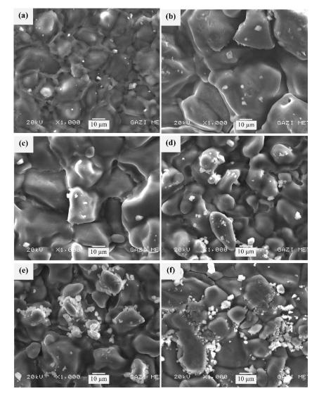
**Figure 3.** Scanning electron microscope (SEM) micrographs of PVA/NH<sub>4</sub>NO<sub>3</sub>/ZnO NSPEs with different ZnO-NP concentrations: (a) NSPE-0, (b) NSPE-1, (c) NSPE-2, (d) NSPE-3, (e) NSPE-4, and (f) NSPE-5.
