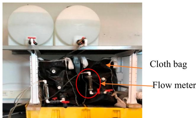
**Figure 1.** Biosand bag filtration setup.
