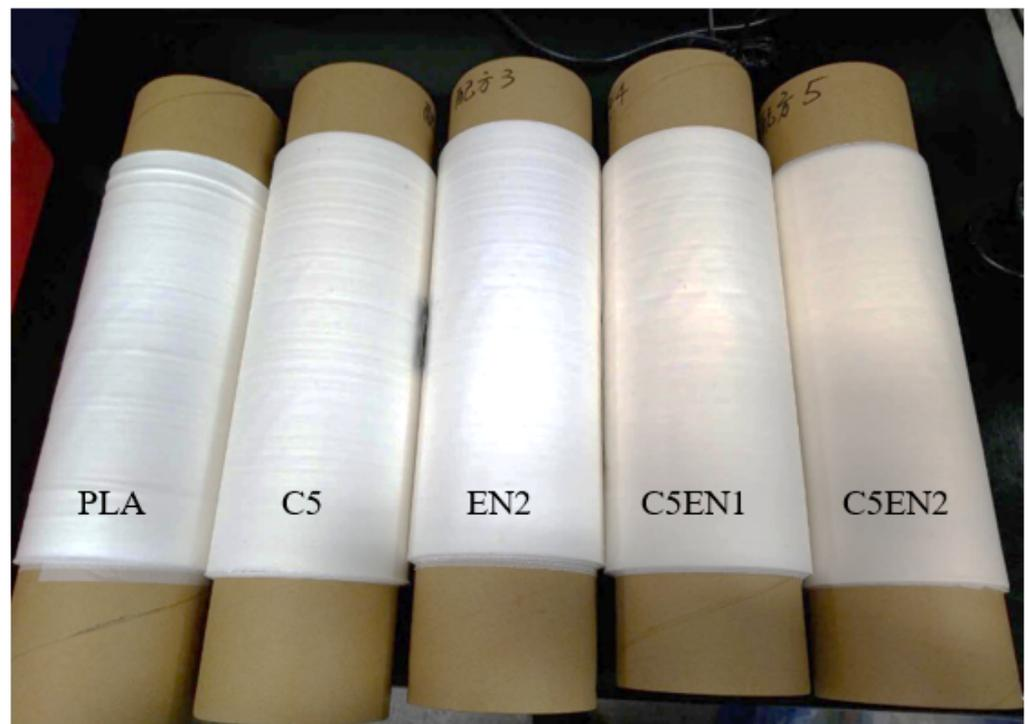
**Figure 2.** Appearance of PLA, C5, EN2, C5EN1, and C5EN2 films. (Film thickness: 30  $\mu\text{m}$ ).
