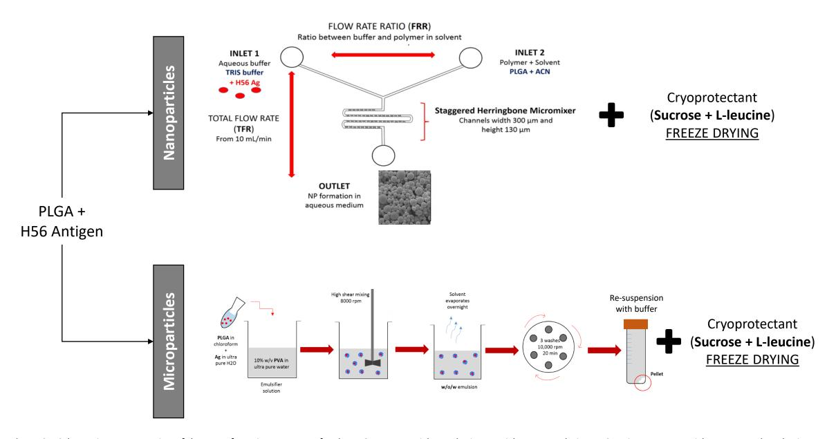
Figure S1. Schematic representation of the manufacturing processes for the PLGA nanoparticles and microparticles encapsulating H56 antigen. Nanoparticles were produced using microfluidics at a TFR 10 mL/min and FRR 1:1 whereas microparticles were prepared using the double emulsion method. Cryoproctants were added post-manufacture and then, particles were freeze dried.
