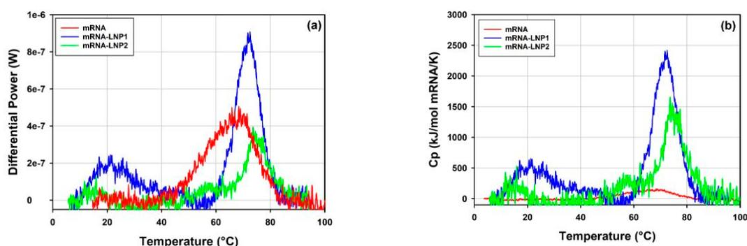
**Figure 15.** Overlays of the DSC traces of mRNA-LNP1, mRNA-LNP2 and free mRNA samples corrected for the instrumental blank and baseline and presented as (a) not normalized differential power and as (b) normalized per mole of mRNA for each sample and expressed as apparent excess heat capacity.
