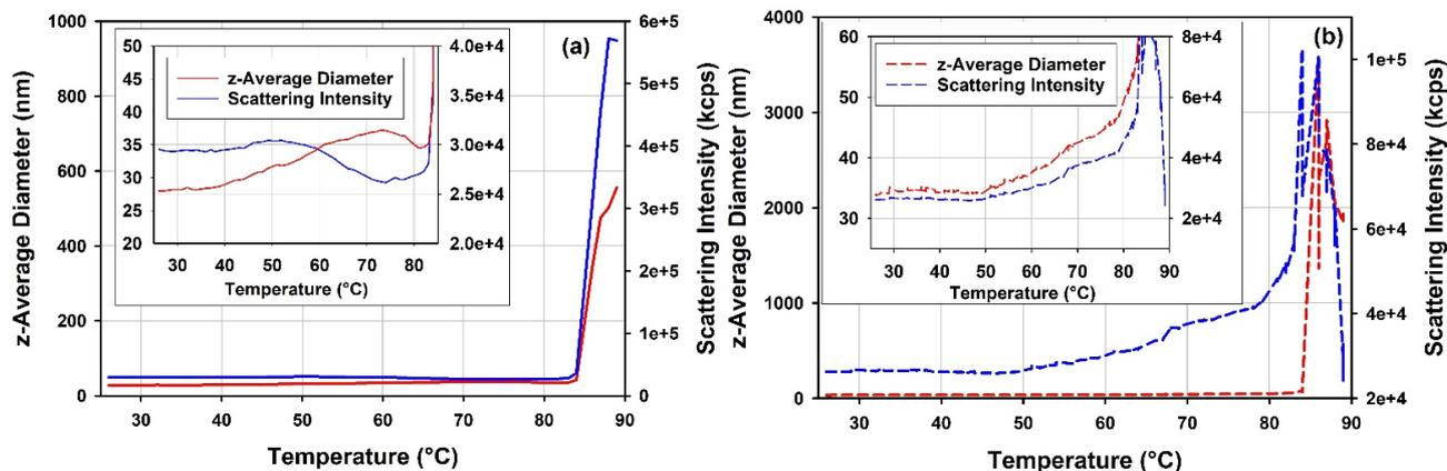
**Figure 12.** DLS thermal ramp data as overlays of the scattering intensities, DRC in kilocounts per second and z—average hydrodynamic diameter in nanometers as a function of temperature for (a) the full rAAV5 and (b) for the empty rAAV5.
