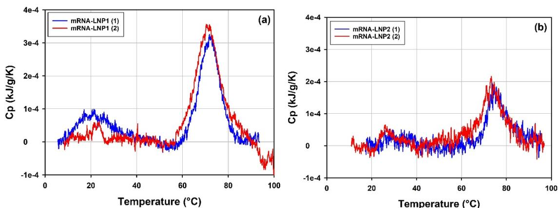
**Figure 14.** Overlays of the thermograms obtained for (a) mRNA-LNP1 and (b) mRNA-LNP2 batch 1 samples. DSC data corrected for the instrumental blank and the baseline and normalized for the total lipid concentration.
