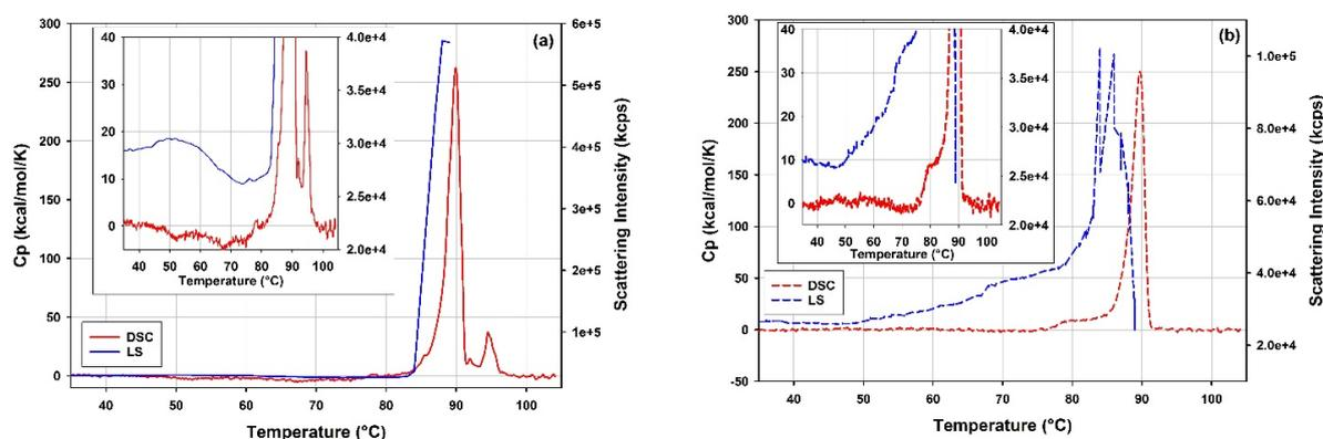
**Figure 11.** Overlay of the DSC and Light Scattering (LS) thermal ramp traces of (a) the full and (b) the empty rAAV5 samples. The inserts show the overlays in the temperature range preceding the main transition. The DSC data are corrected for the instrument blank and the baseline contribution and normalized by the VP protein content in the respective rAAV5 samples. The light scattering data from the thermal ramp DLS measurement is presented as derived count rate, DCR in kilocounts per second.
