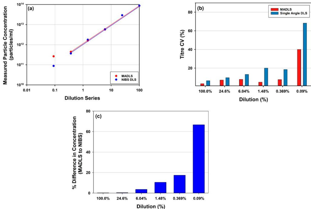
**Figure 5.** Comparison of rAAV5 concentrations measured using single-angle DLS (backscatter) or MADLS: (a) Total viral particle concentration for the sample across the dilution series; (b) Variability across repeat measurement for each dilution; (c) Deviation in concentration value determined with single-angle DLS versus MADLS measurements.
