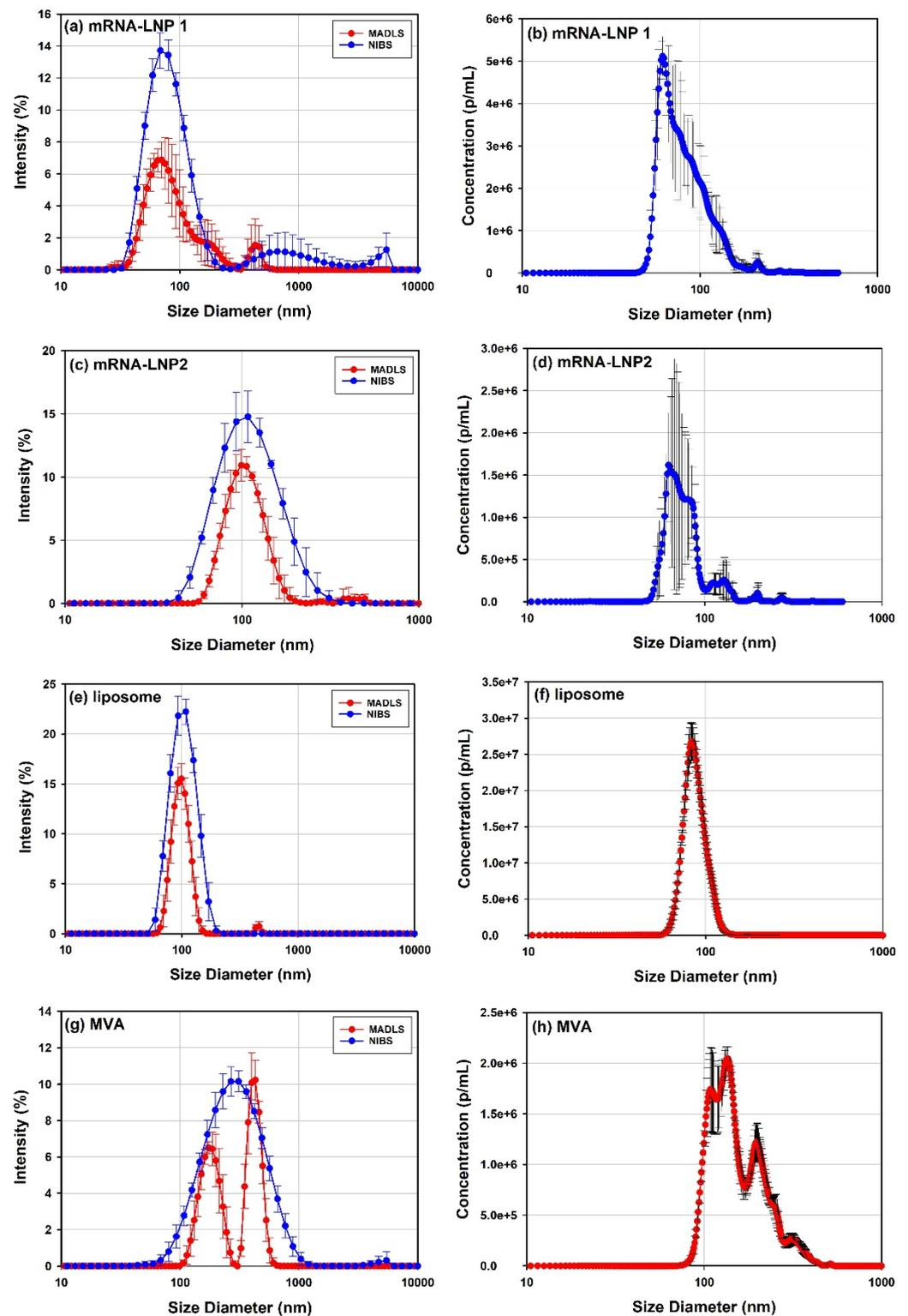
**Figure 2.** Example of size distributions measured with DLS measured through non-invasive back scattering (NIBS) detection and MADLS (a,c,e,g) and NTA (b,d,f,h) are shown for a variety of delivery vectors such as mRNA-LNP 1 (a,b), mRNA-LNP2 (c,d), liposome (e,f) and MVA (g,h) vectors.
