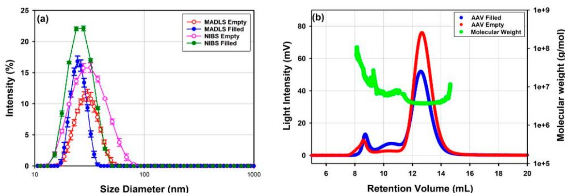
**Figure 3.** (a) Non-invasive backscatter DLS and MADLS intensity PSDs of rAAV5 samples batch 1 that are either full or empty. (b) shows how SEC separation of the same samples ahead of static light scattering detectors increases size distribution resolution compared to MADLS.
