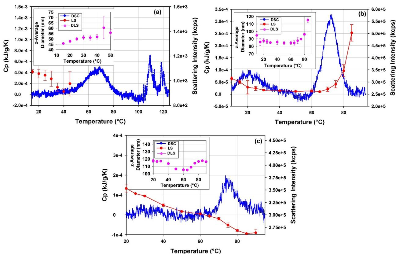
**Figure 16.** DSC thermograms overlaid on DLS thermal ramp data displayed as light scattering intensity vs. temperature for (a) the free mRNA, (b) mRNA-LNP1 and (c) mRNA-LNP2. The inserts present the dependence of the z-average diameter on temperature for the respective samples. To facilitate the comparison, DSC data are shown normalized per mass concentration of the sample, i.e., per gram of mRNA for the free mRNA sample and per gram of total lipids for mRNA-LNP1 and mRNA-LNP2, respectively.
