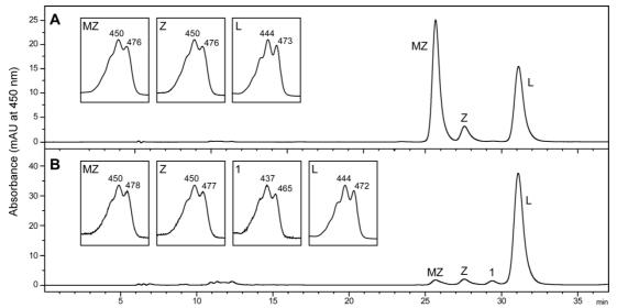
**Figure S1.** Representative chiral HPLC carotenoid profile of a capsule from intervention Group 2. (A) Analysis of the complete content of the capsule (8 mg of *meso-zeaxanthin* (MZ), 1 mg of zeaxanthin (Z) and 6 mg of lutein (L) microcrystals suspended in vegetable oil. (B) Analysis of the vegetable oil separated from the microcrystals (1, unidentified carotenoid).
