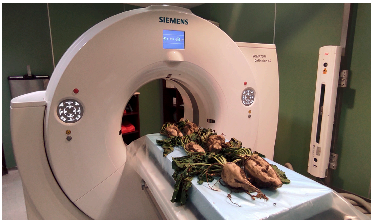
Figure 3. The analysed sugar beet samples in the Siemens CT scanner. The acquisition parameters with a 100 kV tube voltage, with an X-ray dose of 250 mAs, spiral data collection mode with a pitch of 0.4, slice thickness of 0.6 mm, field of view (FoV) of 102 mm, and convolution kernel were I50f. The data collection takes 60–90 s, so the scan did not exceed 10 min for the sugar beet samples analysed. The total number of reconstructed CT images ranges from approximately 1000 to 7000, depending on sample size and resolution.
