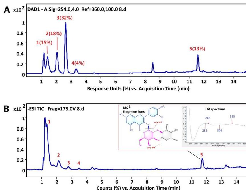
**Figure 1.** (A) UV chromatogram at 254 nm and (B) total ion chromatogram in negative mode of LBPE with the insert graphs of (+)  $MS^2$  fragment ions and UV spectrum of peak 5.
