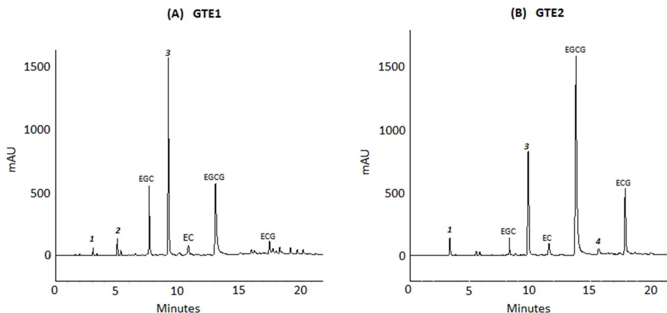
**Figure 2.** Chromatographic separation of catechins from two green tea extracts, GTE1 (A) and GTE2 (B). A binary solvent gradient system with solvent A (1% formic acid in water) and solvent B (1% formic acid in acetonitrile) was used. Identified and quantified compounds: EGC = epigallocatechin, EC = epicatechin, EGCG = epigallocatechin gallate, ECG = epicatechin gallate. Other compounds 1 = gallic acid, 2 = gallocatechin, 3 = caffeine, 4 = gallocatechin gallate.
