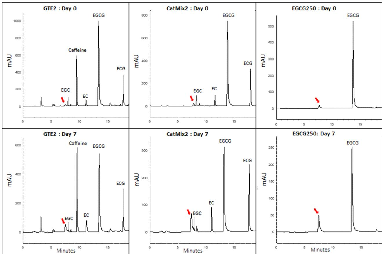
**Figure 6.** HPLC-UV chromatograms of a degradation product formed in catechins-supplemented DHA-rich oils during an accelerated storage test at 30 °C. GTE2 = DHA-rich oil + 450 ppm GTE2, CatMix2 = DHA-rich oil + reconstituted catechins mixture of GTE2, EGCG250 = DHA-rich oil + 250 ppm EGCG. The extracts from EGCG250-supplemented oil injected on HPLC were two times more diluted than the GTE2 and CatMix2 samples to avoid peak saturation. The degradation product is indicated by the arrow.
