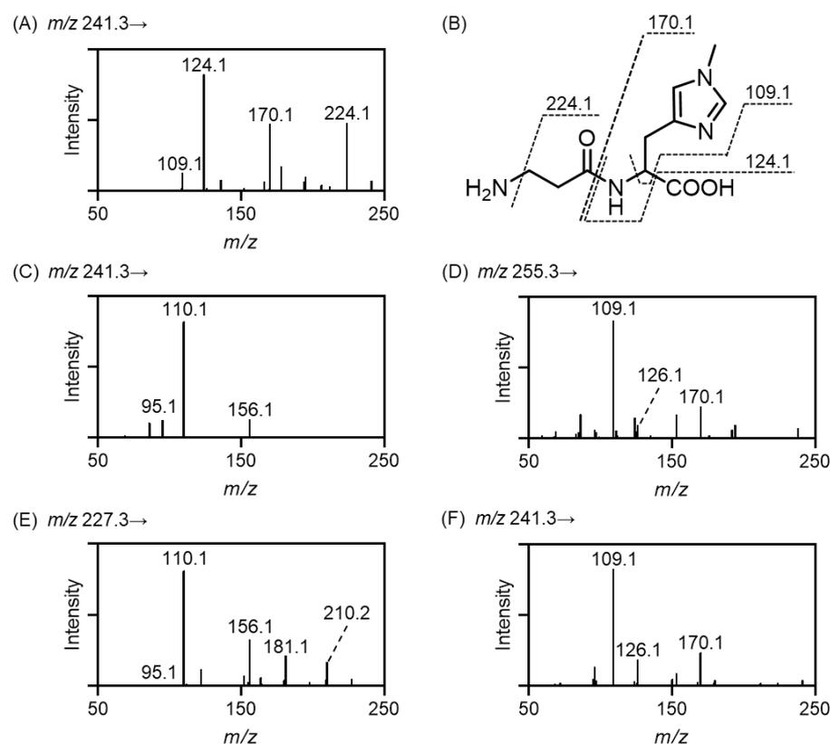
**Figure 1.** MS/MS spectra of IDPs. IDPs were synthesized by the carbodiimide coupling reaction and subjected to HPLC-ESI-MS/MS. MS/MS spectra of balenine (A), homocarnosine (C), homoanserine (D), carnosine (E), and anserine (F) are shown, respectively. Product ions of balenine were assigned as shown in (B).
