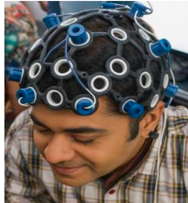
Figure 2. The EEG skullcap designed in-house.
