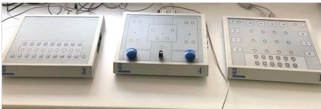
Figure 1. Complex Reactionmeter Drenovac (CRD)-series. In this research, test CRD311 assessing discrimination of simple visual stimulus was solved on the left panel marked with number 3, test CRD411 assessing complex psychomotor coordination was solved on the middle panel marked with number 4, and test CRD11 assessing convergent thinking through solving simple mathematical operations was solved on the right panel marked with number 1. The light stimulus in all tests was presented in small circles on each panel.
