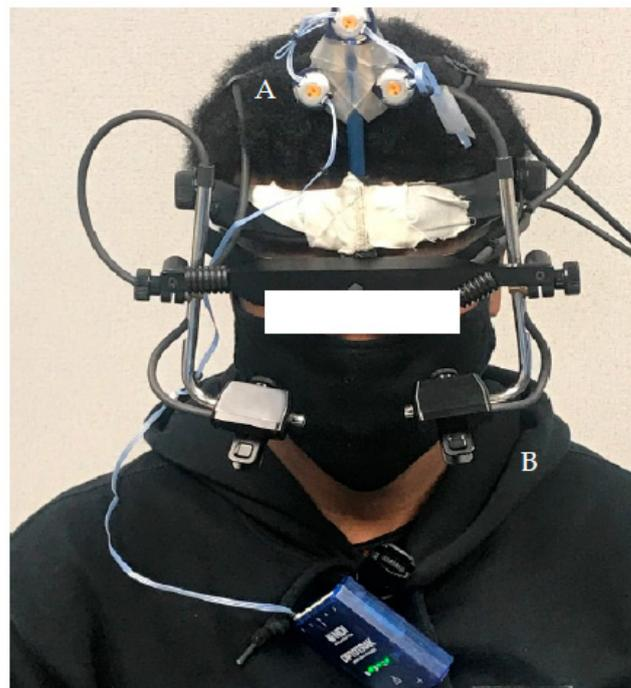
**Figure 1.** Eye-tracker set-up: (A) three infrared markers and (B) the eye-tracker used to capture ocular movement.
