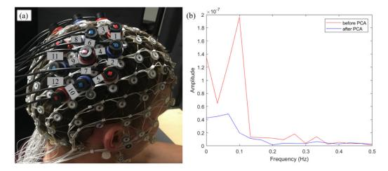
**Figure 1.** (a) NIRS optode arrangement. Red optodes: light sources; blue optodes: light detectors; numbers: channels formed by a source-detector pair; (b) power spectrum density analysis on hemodynamic signals before and after principle component analysis (PCA).
