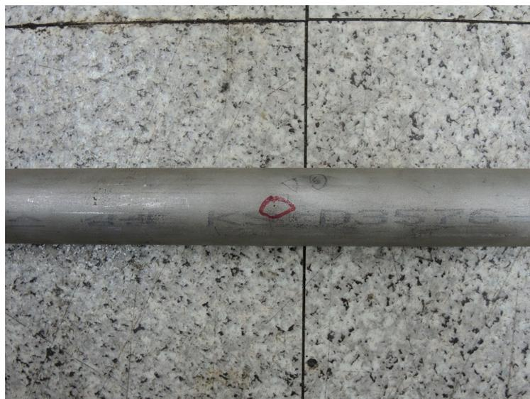
**Figure 6.** A simulated leak orifice of the pipe.
