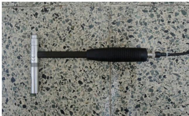
**Figure 8.** An impulse hammer.
