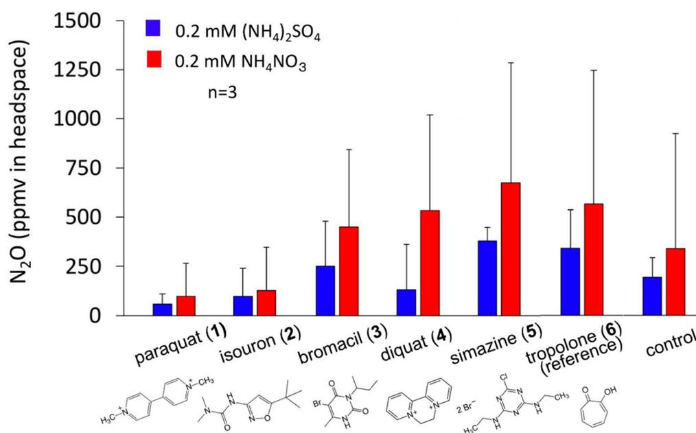
**Figure 4.** Suppression of N<sub>2</sub>O emission from Andisol soil bed by the addition of the Hill reaction-inhibiting herbicides. Incubation was performed for seven days. Bars are standard deviation ( $\pm$  SD,  $n = 3$ ).
