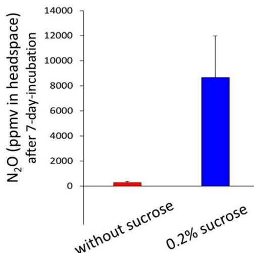
**Figure 2.** Acceleration of N<sub>2</sub>O emission from Andisol soil bed by sucrose supplementation. Effect of 0.2% sucrose supplementation on N<sub>2</sub>O emission from raw soil bed (5.0 g) from the Andisol corn farm placed in a gas-chromatography vial. Bars are standard deviation ( $\pm$  SD,  $n = 5$ ). Soils were also supplemented with 0.2 mM NH<sub>4</sub>NO<sub>3</sub>.
