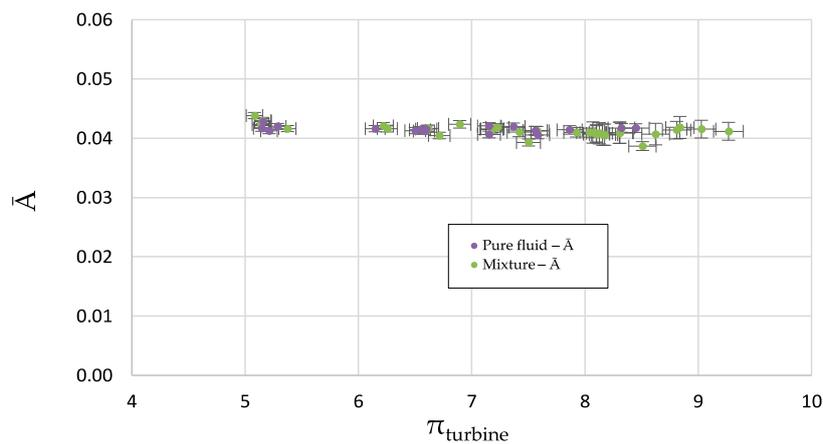
**Figure 3.** The turbine's dimensionless parameter according to the pressure ratio.
