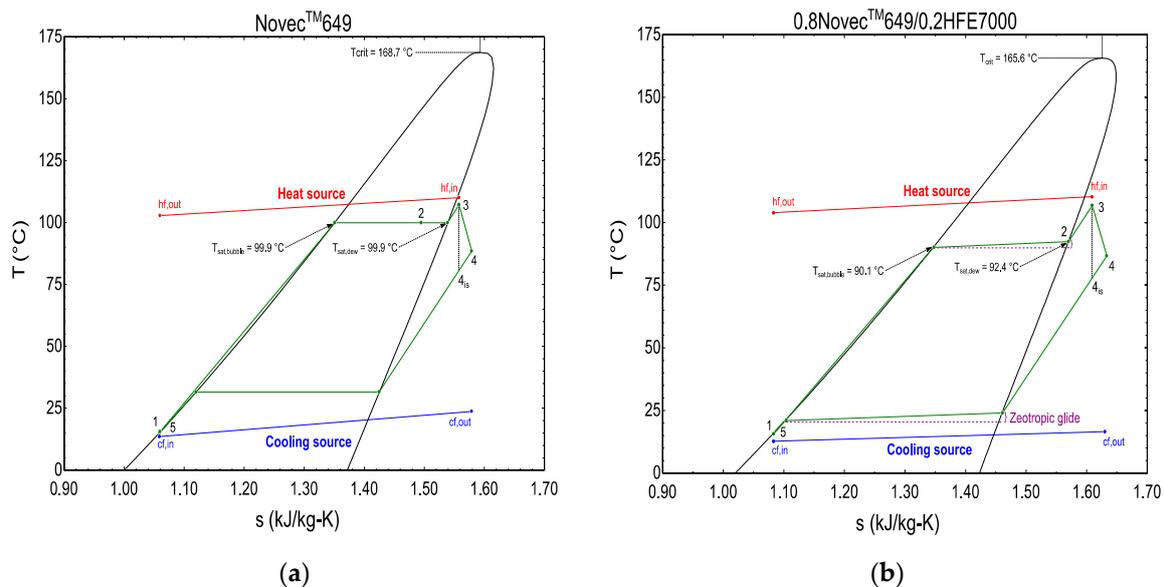
**Figure 8.** The T-s plot of the ORC cycle corresponding to the highest experimental point regarding electrical production: (a) Novec<sup>TM</sup>649; (b) 0.8Novec<sup>TM</sup>649/0.2HFE7000.
