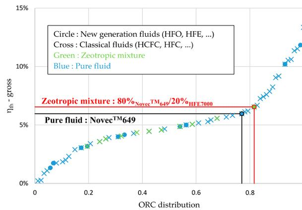
Figure 9. The ORCs’ distribution according to their gross thermal efficiency.
