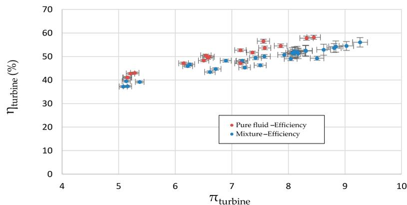
**Figure 4.** The turbine's overall electrical efficiency according to the pressure ratio.
