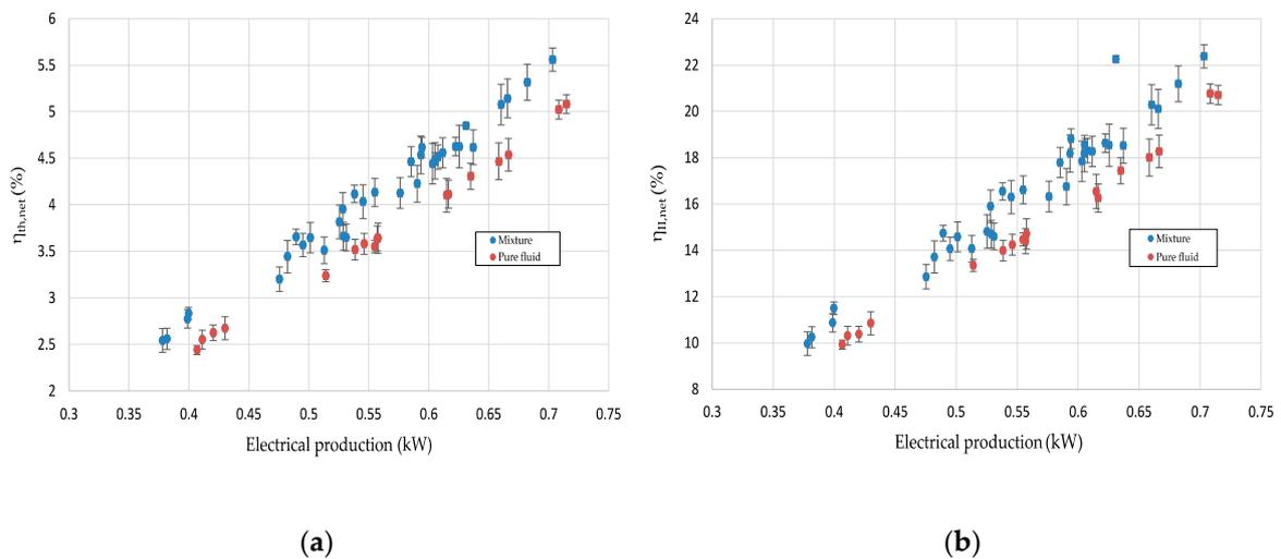
Figure 6. The ORC performance according to electrical production in the pure fluid and the mixture. (a) Thermal efficiency; (b) Second law efficiency.
