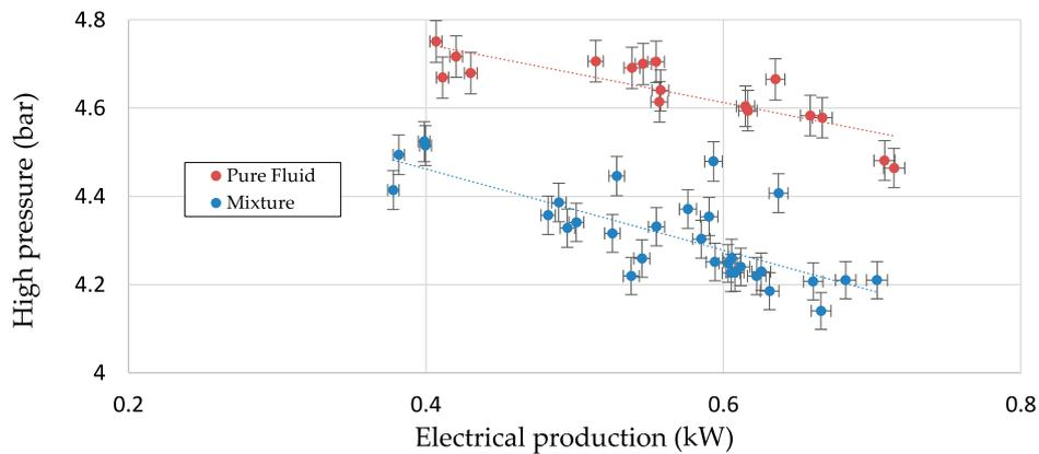
**Figure 11.** ORC performances according to the electrical production in the pure fluid and the mixture.
