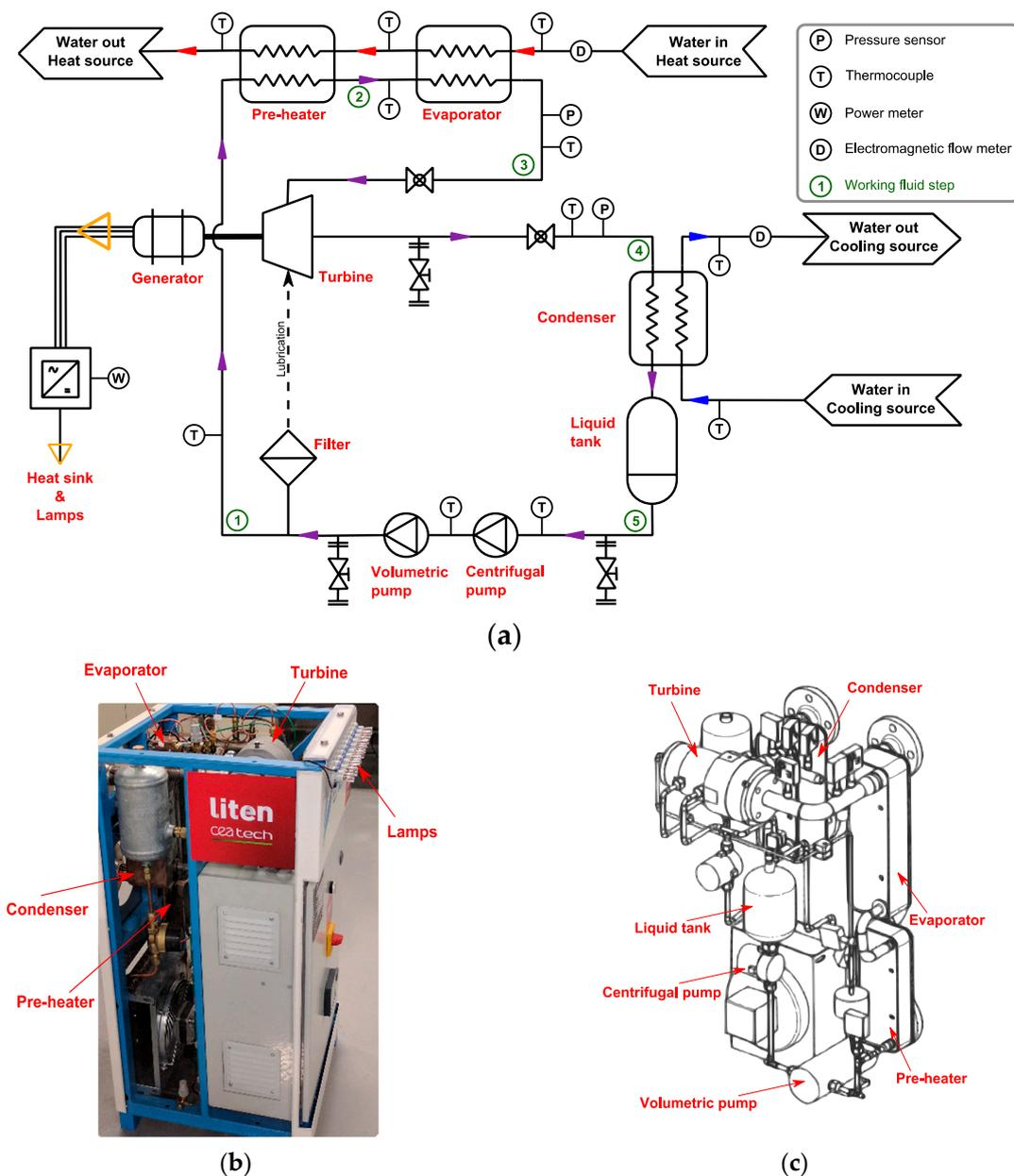
**Figure 1.** The Experimental Organic Rankine Cycle (a) Process Flow Diagram (PFD); (b) Picture; (c) Diagram.
