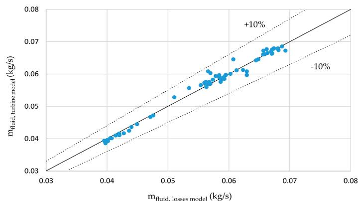
**Figure 12.** The working fluid’s mass flow rate reconciliation between the losses model and the turbine model.
