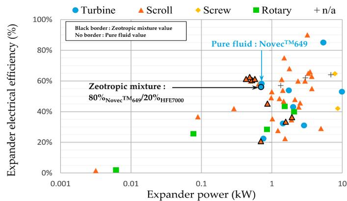
Figure 5. The expander electrical efficiency map for the Organic Rankine Cycle (ORC) up to 10 kW.
