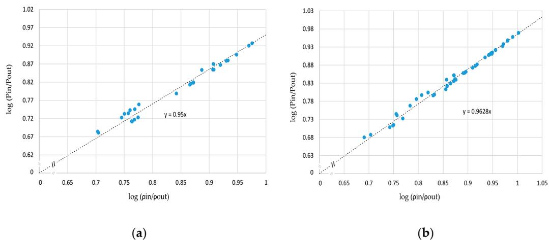
**Figure 2.** The polytropic coefficient in accordance with (a) Pure fluid; (b) Mixture.
