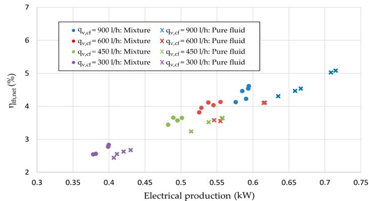
**Figure 7.** The ORC performance according to electrical production in the pure fluid and the mixture (isoparameters).
