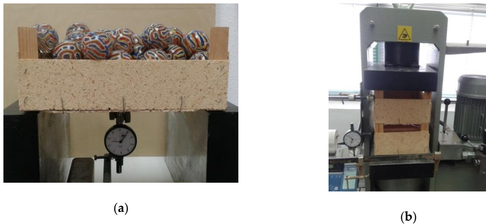
Figure 4. (a) Flexural strength test of the container's base; (b) stacking test.
