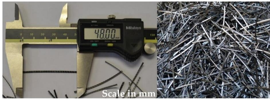
Figure 2. Visual aspect of the polyolefin fibres.
