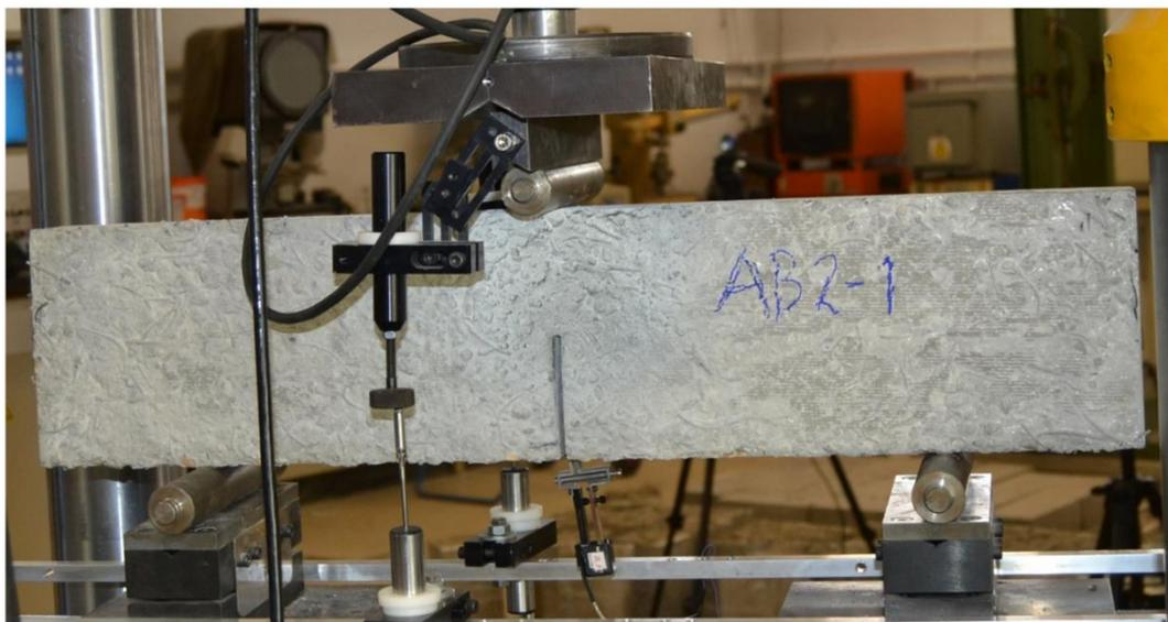
Figure 5. Beam specimen ready for testing.
