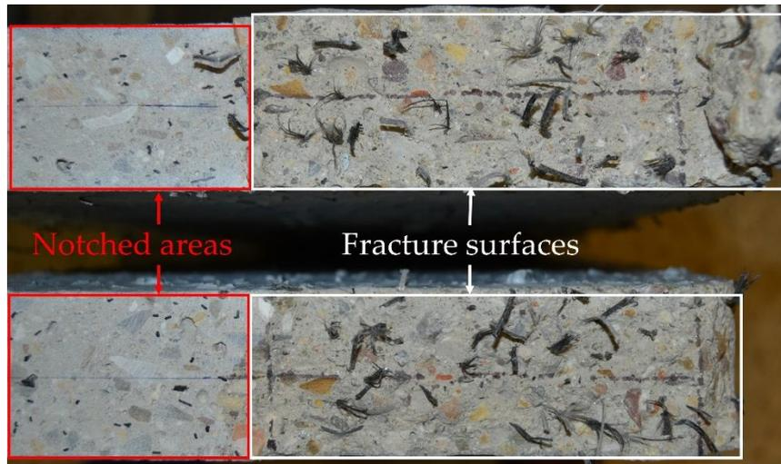
**Figure 8.** Fracture surfaces of one specimen prepared for the fibre counting.
