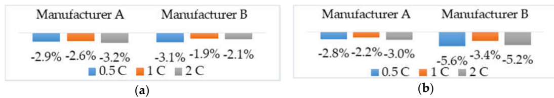
Figure 19. Effects of different charge rates on efficiency change rate of Ni-MH battery modules: (a) change rate of charge efficiency; (b) change rate of discharge efficiency.
