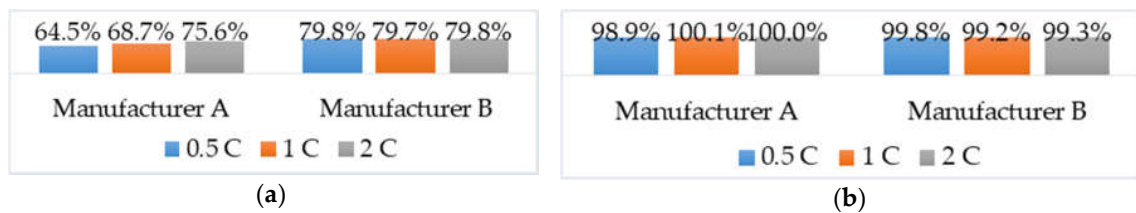
Figure 15. Effects of different charge rates on capacity of Ni-MH battery modules: (a) charge retention rate; (b) capacity recovery rate.
