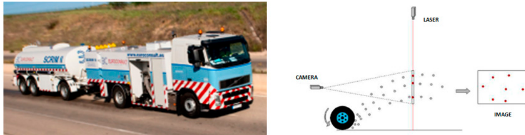
Figure 2. Splash and spray trailer and measuring details.
