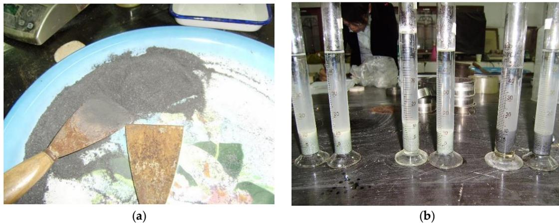
Figure 4. (a) Sample crushing; (b) free expanding rate test.
