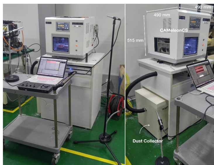
Figure 2. Equipment used to measure and record; noise dust collector and milling machines (CAMEleon CS®).
