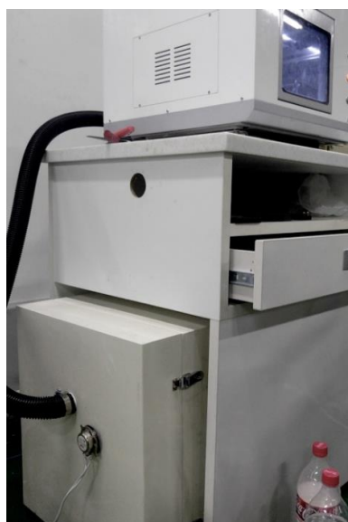
Figure 10. Vibration speaker installed at the dust collector.
