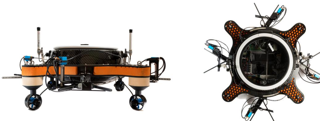
**Figure 6.** The artificial lily pad (aPad) autonomous surface platform, front view (**left**) and top view (**right**).
