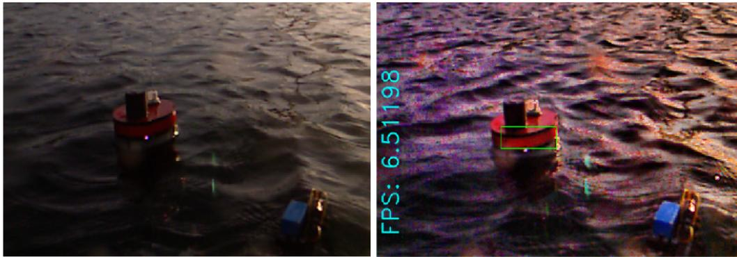
**Figure 19.** Examples of the aPad Kinect RGB image, original (left) and processed (right). The green rectangle superimposed on the camera image represents a bounding box around the derived position of the aMussel top cap used to control the aPad’s approach.
