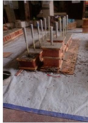
Figure 3. Pullout specimens.
