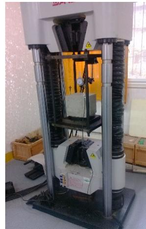
Figure 4. Pullout test setup.
