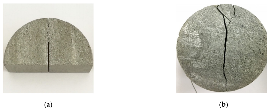
Figure 12. Broken specimens. (a) Broken sample of SCB; (b) Broken sample of BD
