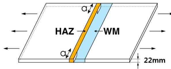
Figure 2. Double-edged through-thickness crack panel with a crack in the heat-affected zone (HAZ).
