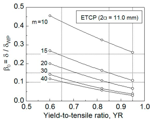
**Figure 4.** Monographs of equivalent CTOD ratio  $\beta_0$  for double-edged, through-thickness crack panel (ETCP) with a reference crack length of  $2a = 11$  mm.
