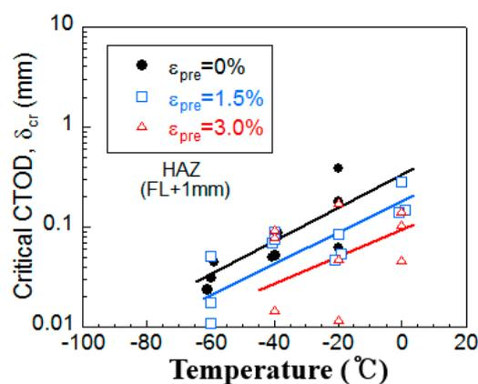
Figure 3. Effect of pre-strain on ductile-to-brittle transition temperature [19].
