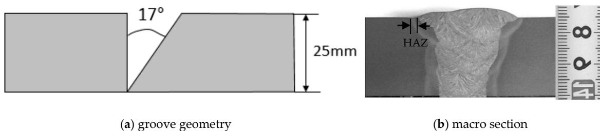
**Figure 1.** Groove geometry and macro section of the weld joint.
