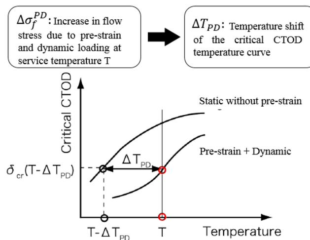
Figure 7. Temperature shift of fracture toughness  $\Delta T_{PD}$  in pre-strained and dynamic conditions.
