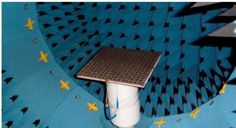
**Figure 22.** Radiated gain measurement of the  $16 \times 16$  array antenna made with StarLab Antenna Measurement Systems-Satimo©.
