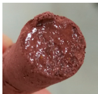
Figure 6. Accumulation of the polymer emulsion on the surface.
