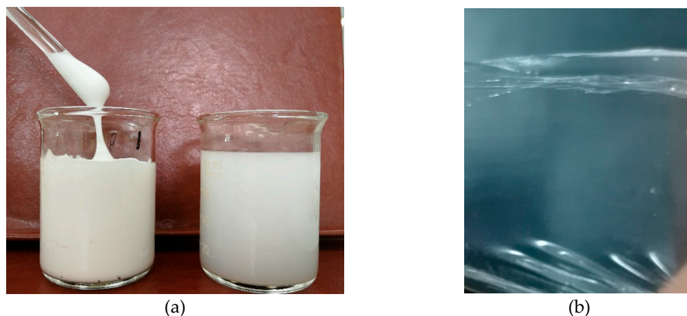
Figure 1. Different states of the aqua-dispersing-nano-binder (ADNB) polymer emulsion: (a) initial state (left), dispersed in water (right); (b) after water evaporation, an elastic film is generated.
