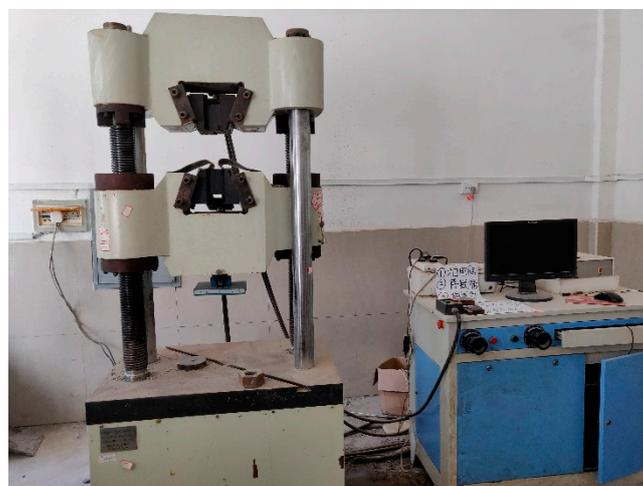
**Figure 4.** Electro hydraulic servo universal testing setup.
