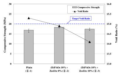
Figure 7. Compressive strength of porous concretes produced with (D)PAOs and zeolite.
