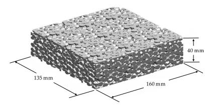
Figure 3. Test specimen size of the porous concrete.
