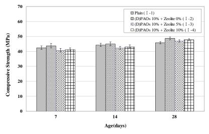
Figure 6. Compressive strength of mortars produced with (D)PAOs and zeolite.
