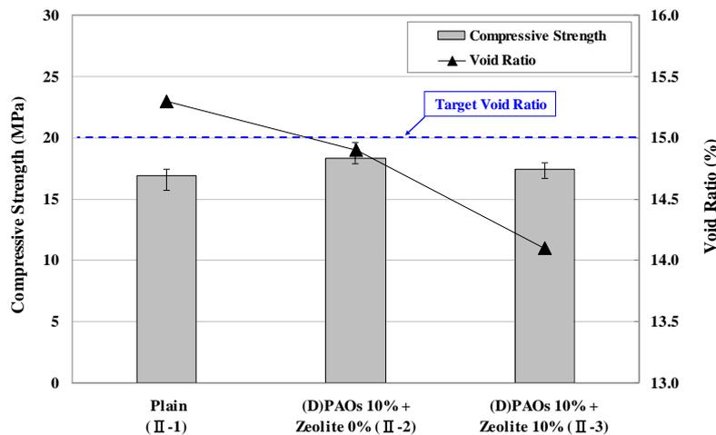
Figure 7. Compressive strength of porous concretes produced with (D)PAOs and zeolite.
