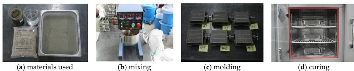
**Figure 2.** Test specimen production of the mortar produced with (D)PAOs and zeolite.
