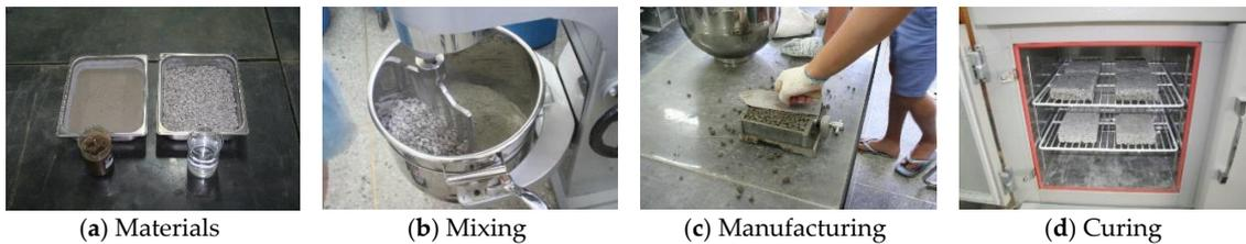
Figure 4. Test specimen production of the porous concrete produced with (D)PAOs and zeolite.
