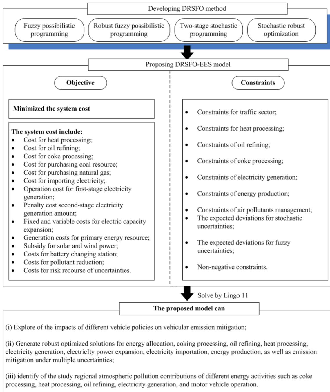
**Figure 2.** The schematic diagram of dual robust stochastic fuzzy optimization—energy and environmental systems (DRSFO-EES).
