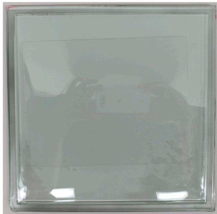
Figure 10. Glass sample sealed using the optimized fabrication conditions.
