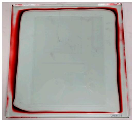
**Figure 3.** Liquid penetrant examination for the basic experiment.
