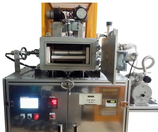
**Figure 1.** Schematic and real picture of microwave heating chamber.
