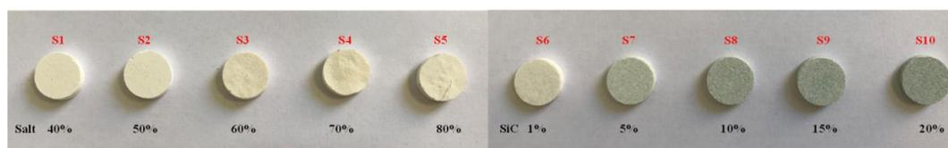
Figure 1. Visual observations of composite PCMs after sintering.
