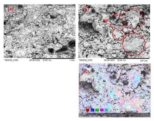
**Figure 5.** SEM images of Sample S8 after 100 thermal cycles: (a)  $100 \times$ ; (b)  $500 \times$ ; (c) EDS mapping,  $500 \times$ .
