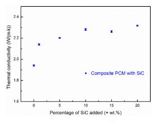
**Figure 2.** The thermal conductivity of composite PCMs with different SiC contents using a mass ratio of salt to MgO of 60:40.
