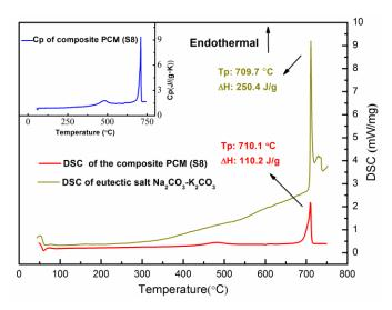
Figure 8. DSC and Cp curves of the composite PCM (Sample S8).
