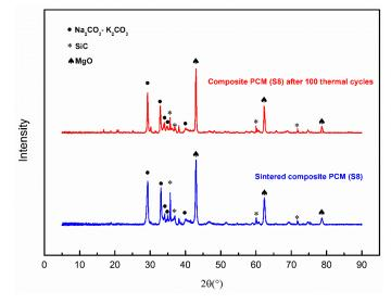
Figure 7. XRD patterns of Sample S8 with and without 100 thermal cycles.
