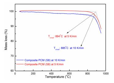
Figure 9. TG curve of the composite PCM.
