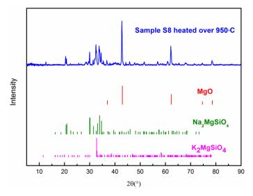
Figure 10. XRD Patterns of composite PCM (S8) heated over 950 °C.
