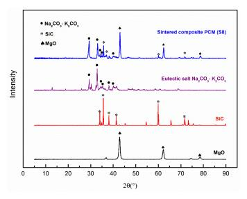
Figure 6. XRD Patterns of the composite PCM and individual components.
