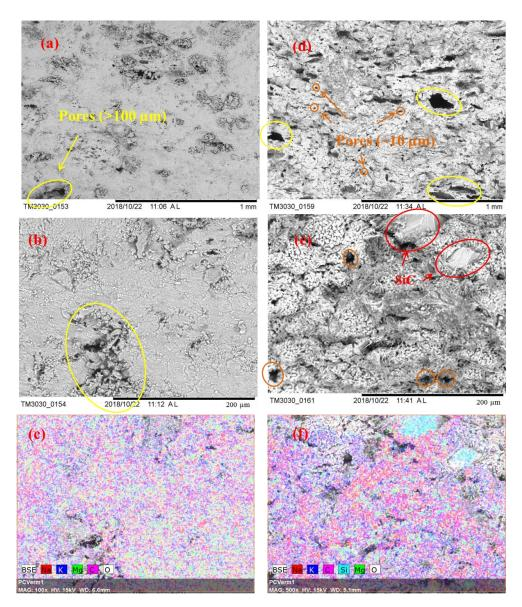
**Figure 3.** SEM images for Sample S3: (a) 100×; (b) 500×; (c) EDS mapping, 500×; SEM images for Sample S8: (**d**) 100×; (**e**) 500×; (**f**) EDS mapping, 500×.
