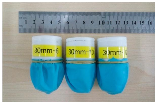
**Figure 14.** Three CTSA-II hands with different numbers of pin assemblies.
